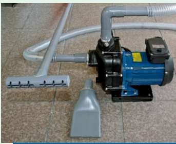
Pump for pond cleaning
